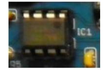
Note that you may need to form the leads on the ICs to align with the socket. If this is necessary, do so carefully to avoid breaking the IC leads.
